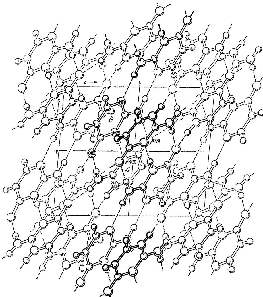
Fig. 5. The structure viewed along the *b* axis. The dashed lines represent hydrogen bonds.
