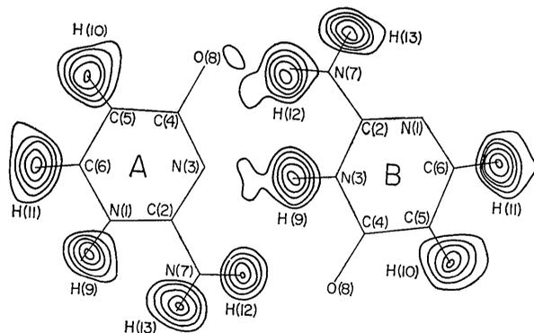
Fig. 2. The composite of the final difference maps in the respective least-squares planes of the heavy atoms of molecules *A* and *B*, in which the hydrogen contributions were omitted from the  $F_c$ 's. Contours are at intervals of  $0.1 \text{ e.}\text{\AA}^{-3}$  beginning with  $0.1 \text{ e.}\text{\AA}^{-3}$ .
